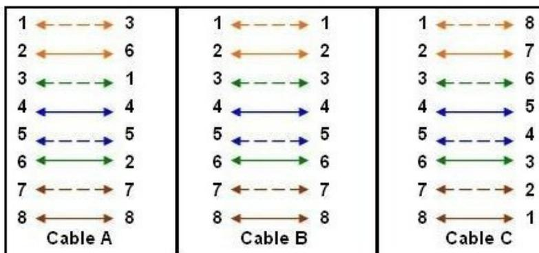
Refer to the exhibit. Which answer correctly identifies the pinout of the UTP cables labeled Cable A, Cable B, and Cable C?
