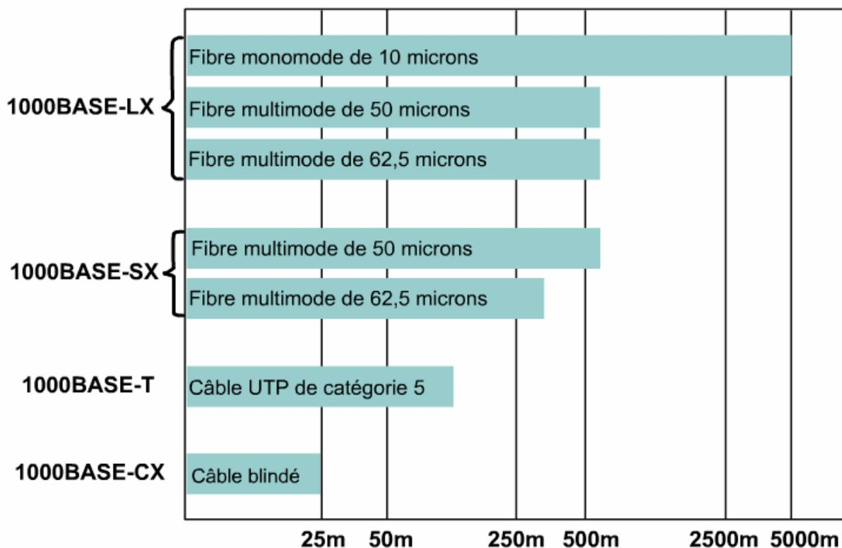
In a departure from both [10BASE-T](#) and [100BASE-TX](#), 1000BASE-T **uses all four cable pairs for simultaneous transmission in both directions** through the use of echo cancellation and a 5-level [pulse amplitude modulation](#) (PAM-5) technique
